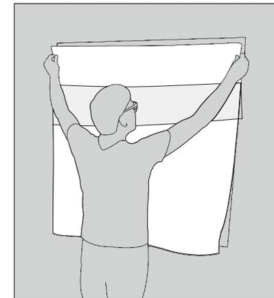
Align the Squid® with the top of the window and press the textile gently onto the glass. Take out the remaining backing paper little by little, by section of  $\pm 15$  cm each, while pressing gently the fabric onto the window from top to bottom and from the middle to the side.
