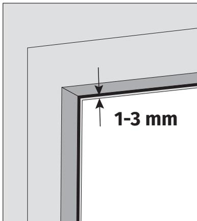
For best results, it is recommended to leave a 1-3 mm gap between the silicon joint and Squid<sup>®</sup>.
