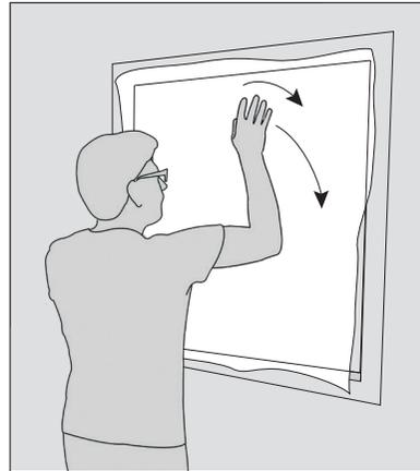
Then let it fall again smoothly onto the window, while accompanying it with your hand or with the squeegee. Never try to push out bubbles or creases by pressing with the squeegee because this would cause permanent deformations in the fabric.
