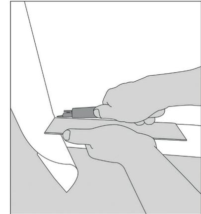
Place the squeegee next to the window silicon joint, with the cutter on the inside. Carefully cut to remove the excess, with a regular movement using strong pressure and a sharp angle. Use a new blade every 2 meters and for every corner, in order to avoid tearing the yarn.
